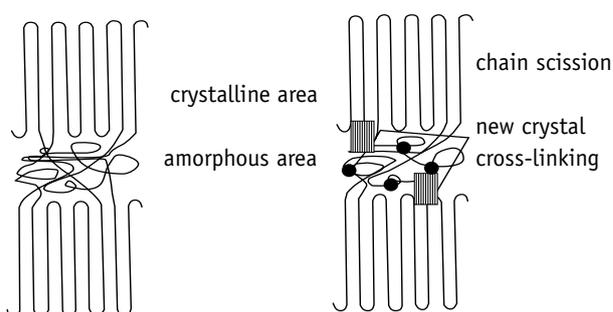
**Figure 1: Effect of irradiation cross-linking on the morphology of a non-irradiated and an irradiated semi-crystalline polymer**
