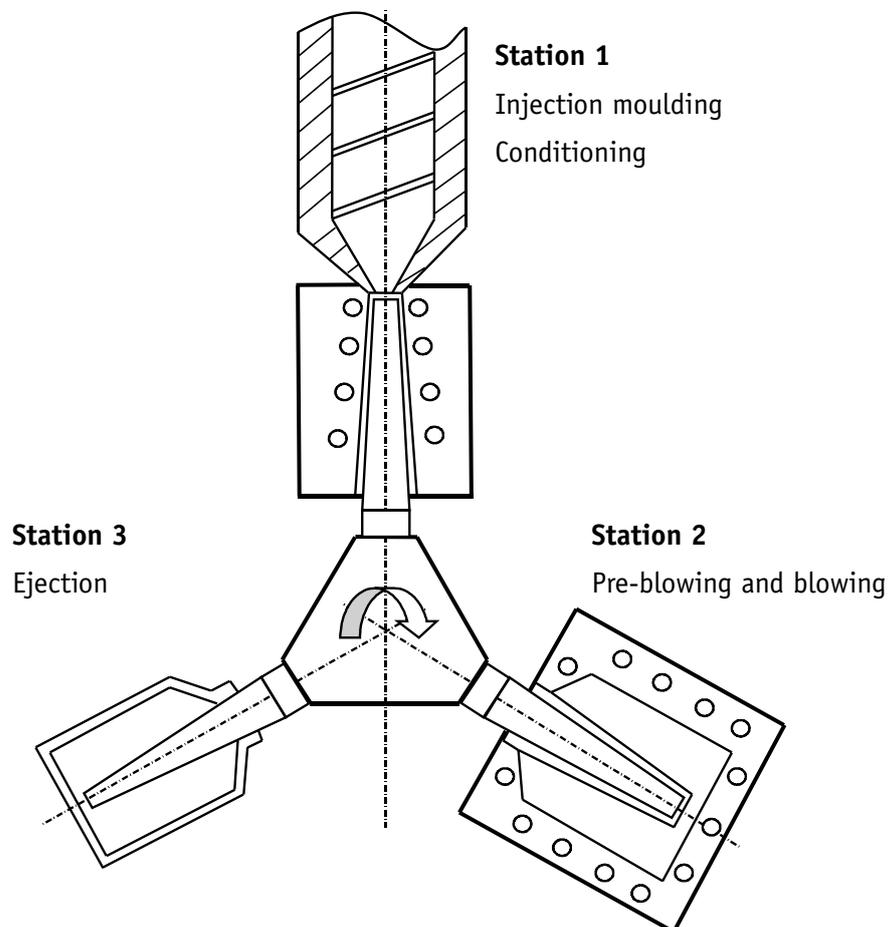
Figure 1: Injection blow moulding
