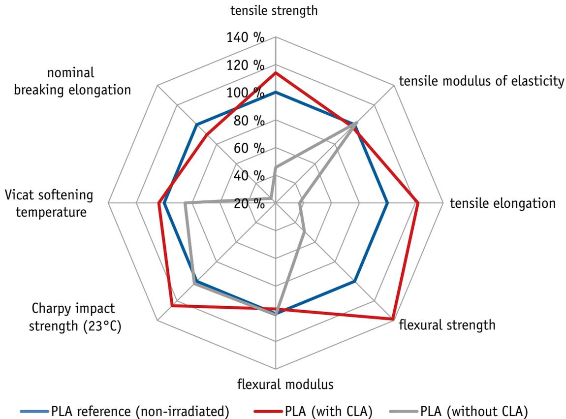
Figure 2: Effects of irradiation on the characteristics of PLA
