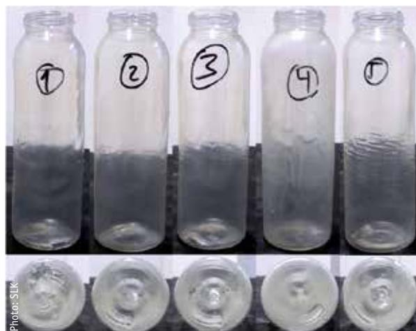
**Figure 2: Injection blow moulded baby bottles made from bioplastics (from left to right: Bio-PE, PLA, PBS)**
