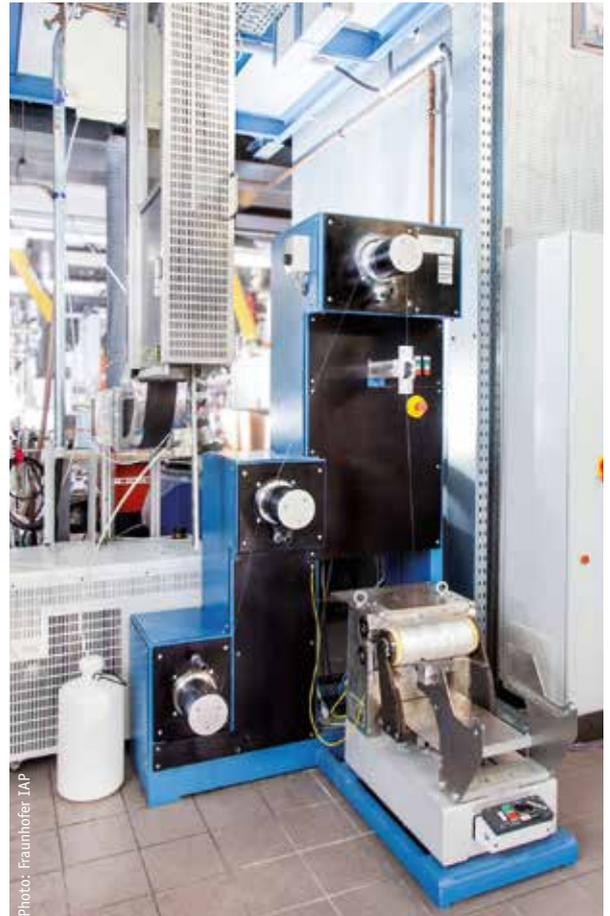
**Figure 2: Fourné melt spinning machine**
