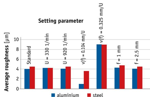
**Figure 2: Average roughness of Ingeo 3251D in dependence on the setting parameters**
