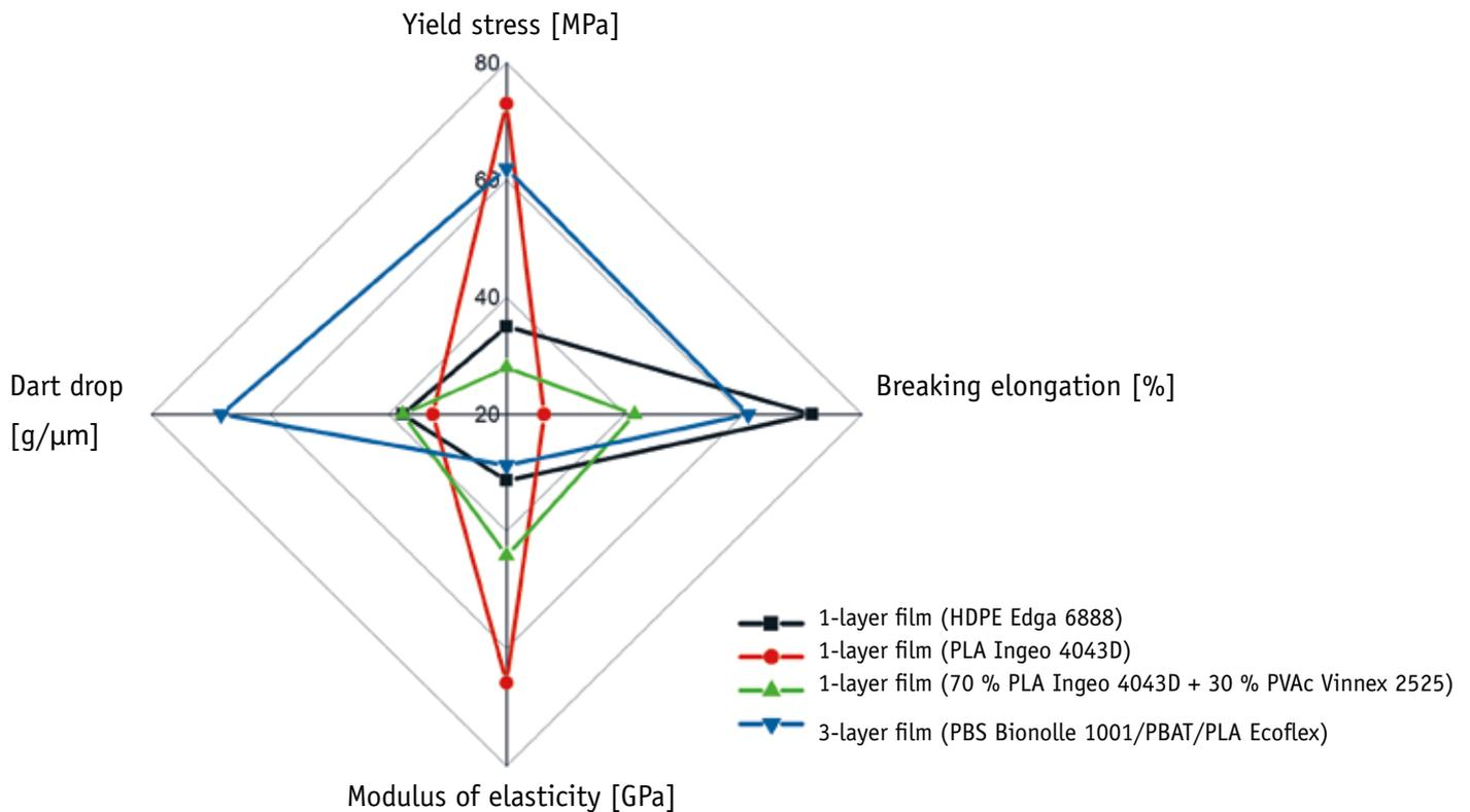
**Figure 2: Comparison of the characteristics of modified and non-modified bioplastic films**
