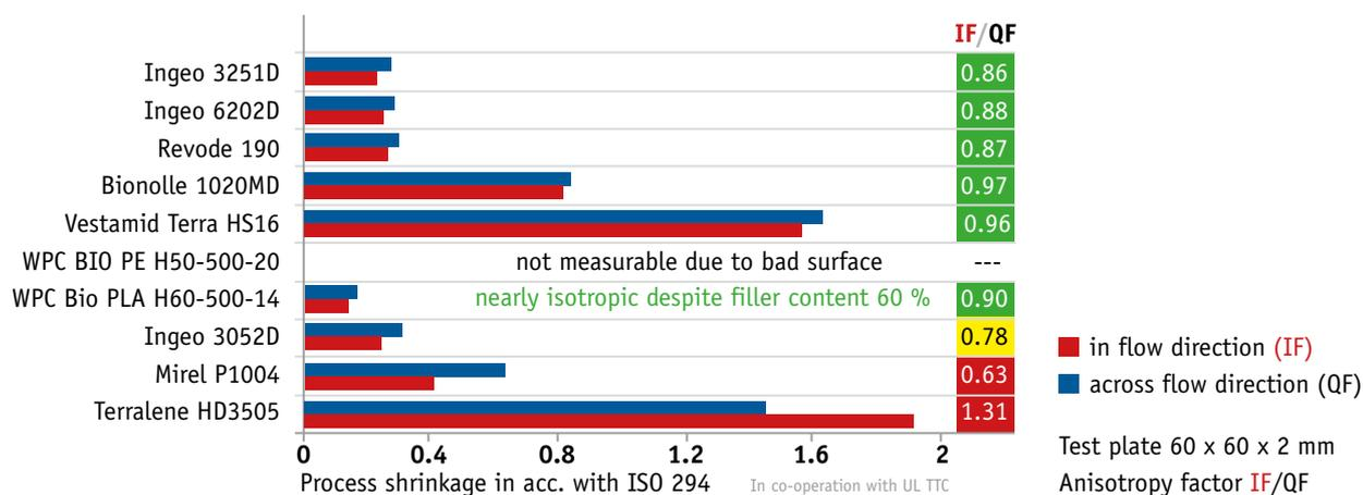
Figure 3: Shrinkage and distortion of bioplastics
