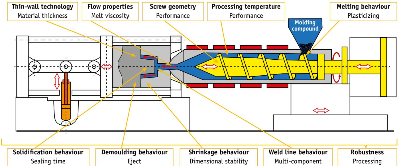
Figure 1: Factors which affect the injection moulding process
