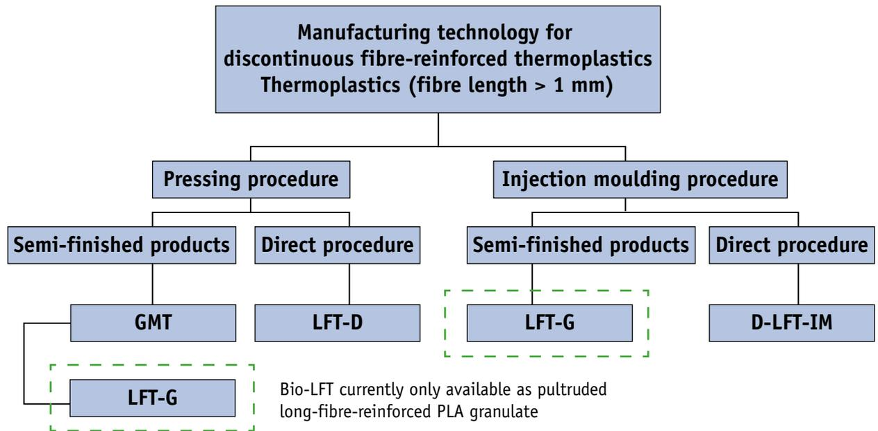
Figure 1: Structure of manufacturing technologies for long-fibre-reinforced thermoplastics
