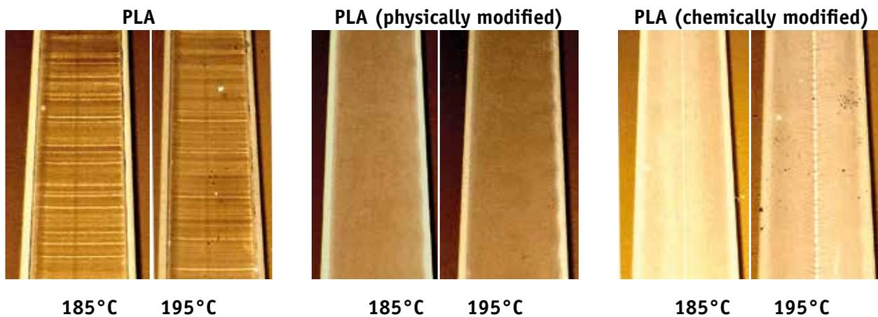
**Figure 2: Extruded profiles from non-modified and modified PLA**
