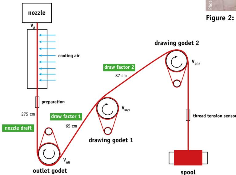
**Figure 1: Filament yarn course in the spinning process**
