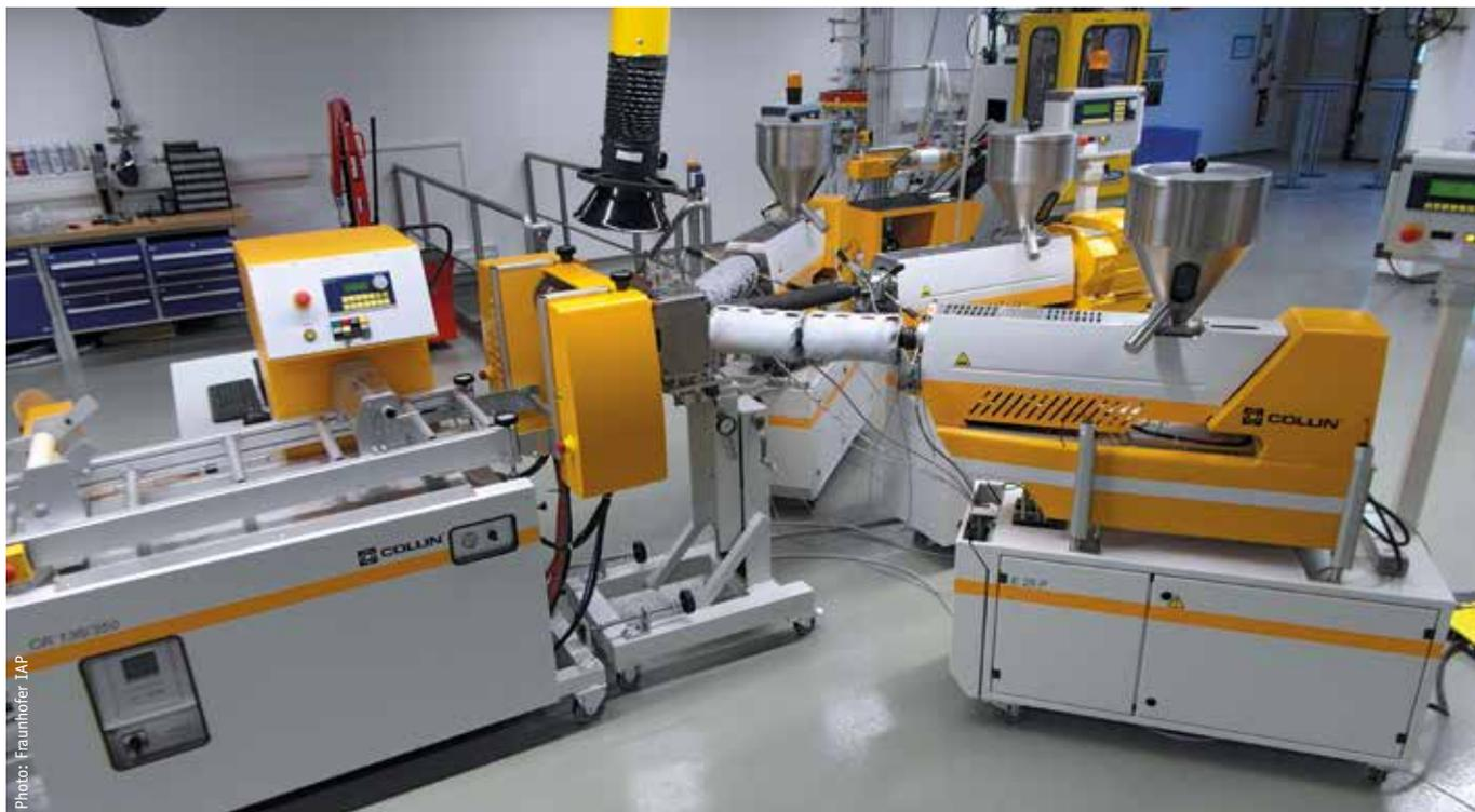
**Figure 1: Three-layer film extrusion system**
