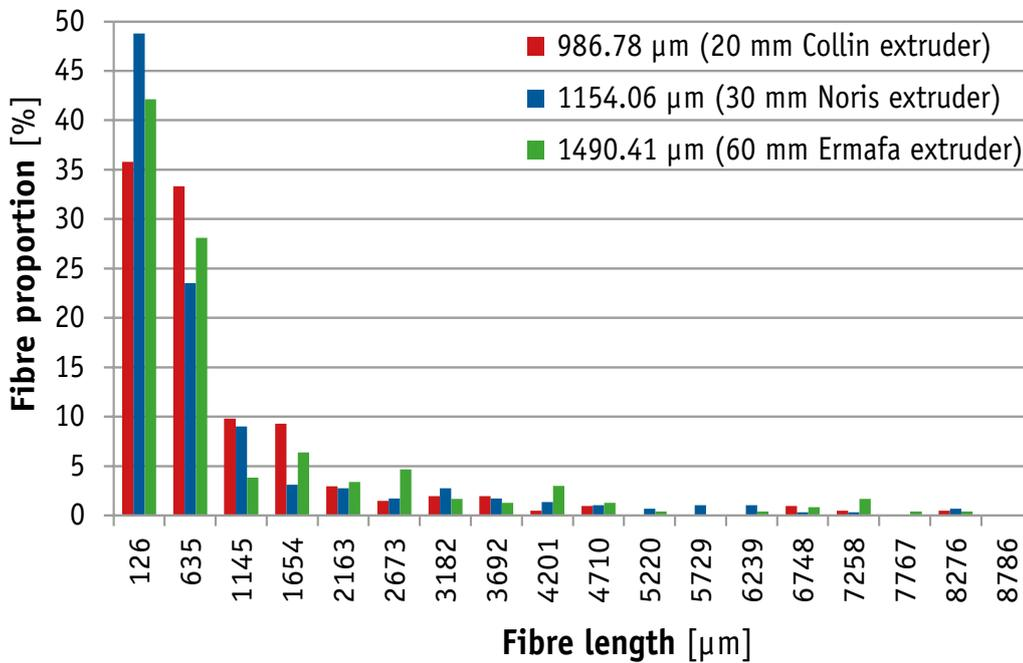
Figure 2: Fibre-length distribution and average fibre length in dependence on the screw diameter
