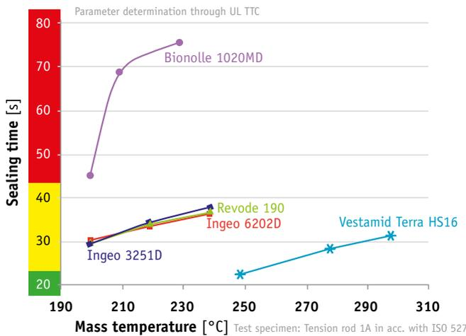
**Figure 4: Sealing times for bioplastics**
